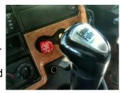
These failures are not a warranty issue as the operating instructions are clear that the operator of the equipment should use the clutch while shifting gears.
