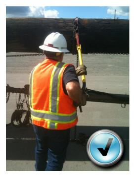
Please note: the hand positioning keeps your hand from slipping off and also allows the driver to stand erect and keep his back straight. Additionally, it ensures his/her face and body are never over the winch bar.
